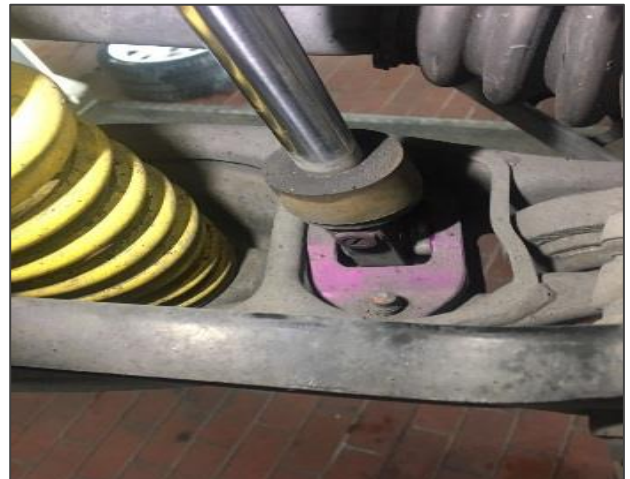
Abb. 5: Falsche Befestigung Figure 5: Wrong mounting
