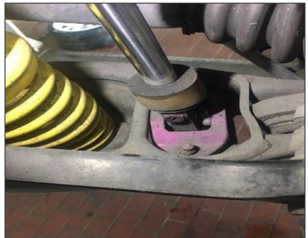
Abb. 5: Falsche Befestigung Figure 5: Wrong mounting
