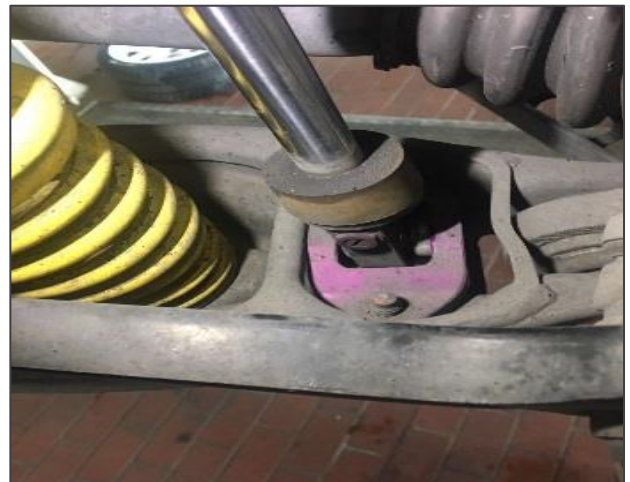
Abb. 5: Falsche Befestigung Figure 5: Wrong mounting
